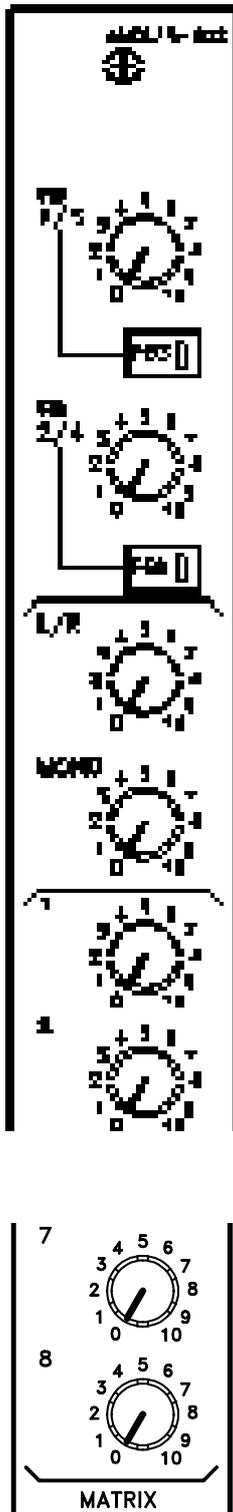
Either 8 or 16 mono subgroup modules may be fitted in Q2. If 16 are fitted, routing is paired, with active pan across the group buses at all times. For 8 modules, routing is individually selected, with pan only switched in across odd and even groups as required.
