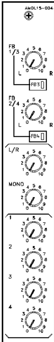
The LCR Subgroup Output module has three outputs (for the left, centre and right outputs from each group). It may be used with either the normal input module or the dedicated LCR input module.
