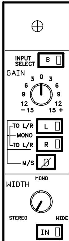
As an option, in place of a standard input, a stereo effect return input may be fitted. The effect return section may be controlled by the VCA master, if VCA/Mute subgrouping is fitted to the console.
