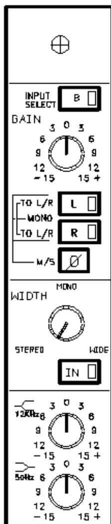
The effect return VCA master is only fitted to consoles with the optional VCA Grouping inputs. The effects return section may be controlled by the VCA masters.
