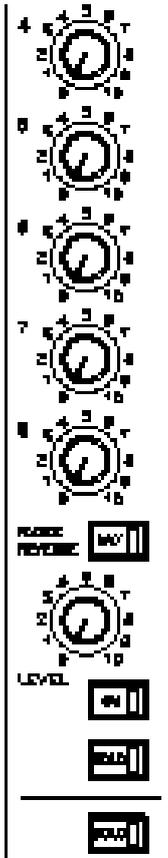
5 Adjusts the level of the GROUP signal fed to MATRIX bus 5.
