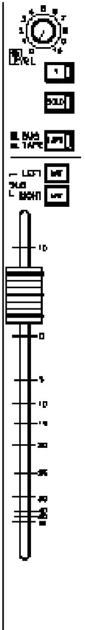
bus, and similarly for hard right. When the pan is in the centre, equal signal, approximately 4.5dB down, is fed to both left and right buses.
