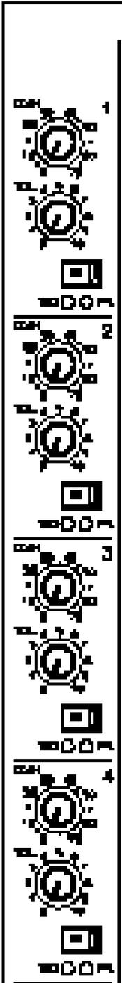
Six microphone inputs are available on this dual width module. Individual gain and level controls and an ON switch are available to each input.
